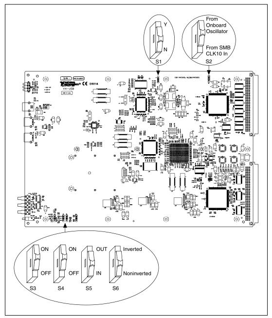
Figure B-1. VXI-USB Default Configuration Settings
